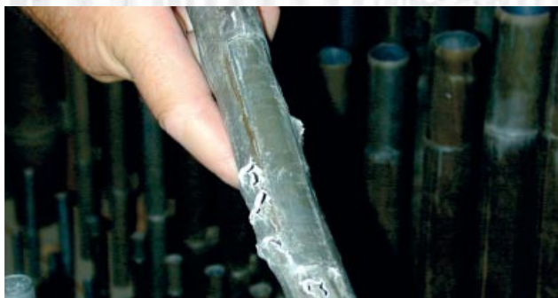
Winded: many lead organ pipes in Europe, such as this one, are disintegrating.
